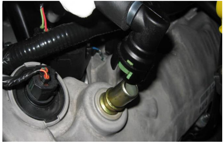
Step 7: Removal of one side of PCV hose from valve cover
