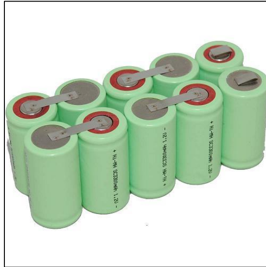
Figure 3: Inside of a 12V battery pack
