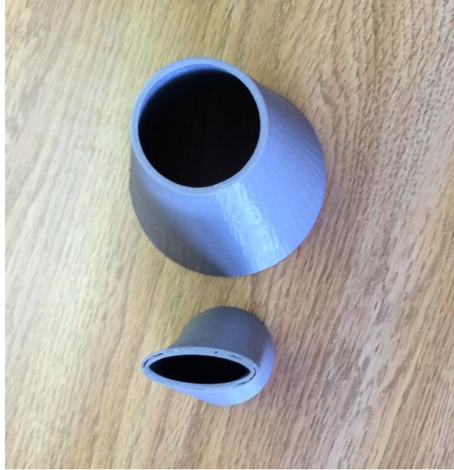
Figure 27: Housing and Nozzle Top View
