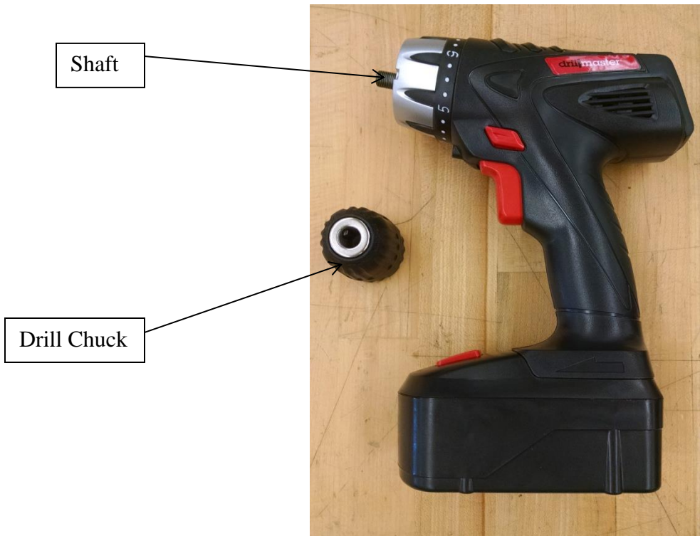
Figure 3: Drill with Detached Chuck
