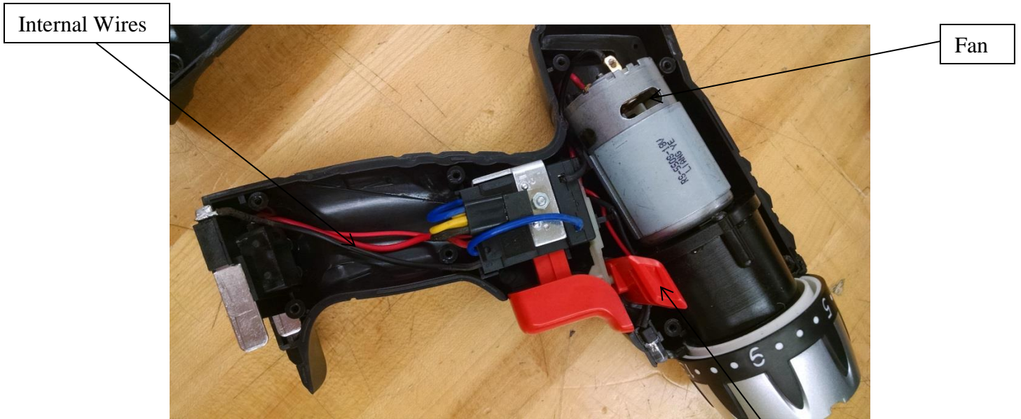
Figure 5: Internal Layout of Drill (Left Housing)
