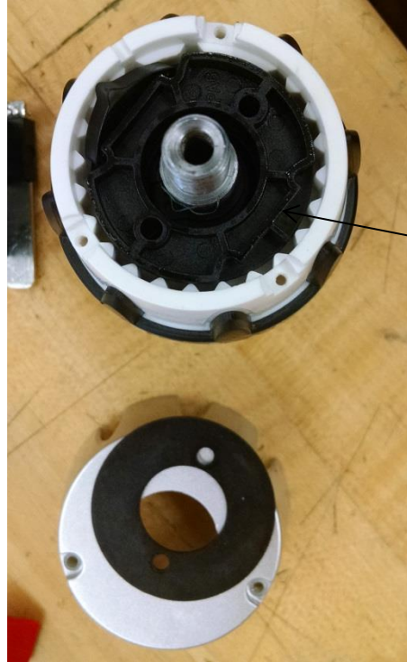
Figure 9: Gearbox with Removed Cover and Torque Ring
