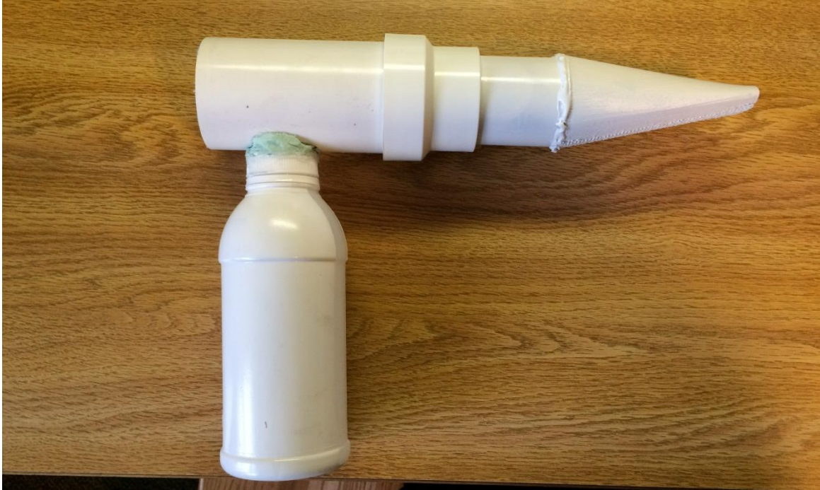
Figure 53: Housing, Nozzle, and Collection Bin Side View
