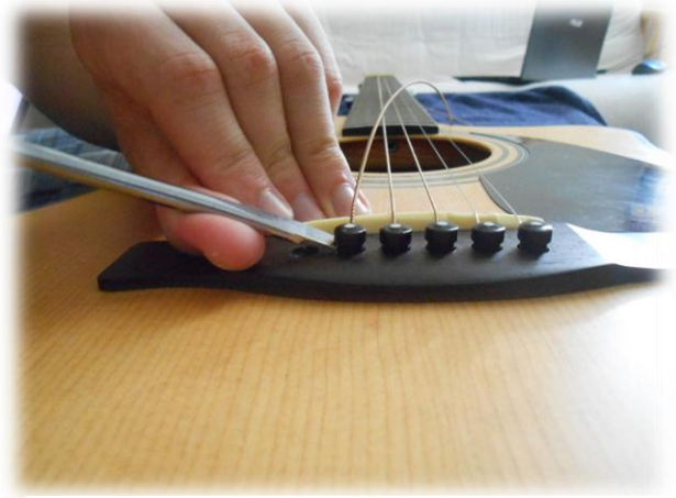
Notice the thumb being used as a fulcrum to get leverage for the screwdriver.
