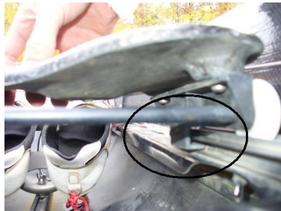
Figure 8: Seat Properly hooked into the tracks
