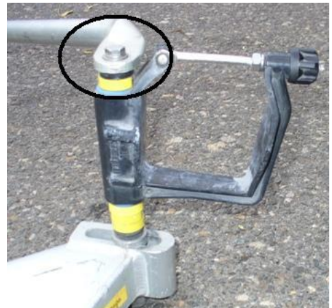
Figure 12: Top nut on the Oarlock
