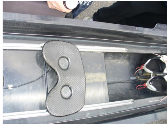
Figure 7: Orientation of seat on tracks
