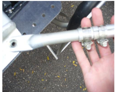
Figure 11: Attaching the backstay
