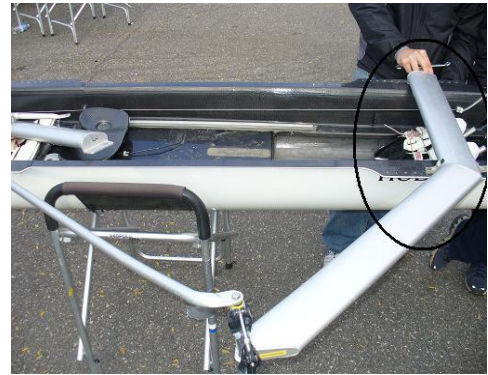
Figure 9: Mounting the rigger
