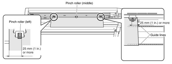
While keeping the material stretched taut, raise the sheet loading levers to secure the material in place.
