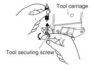
Press the pin and remove the blade from the blade holder.
