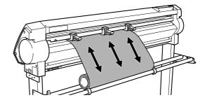
Position the left and right pinch rollers as shown in the figure, and position the middle pinch roller at the center between the left and right pinch rollers. If a grit mark is present between the left and right pinch rollers, position the middle pinch roller above the corresponding grit roller.
