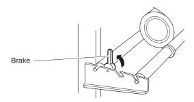
Pull out the material from the roll and pass it through the unit.
