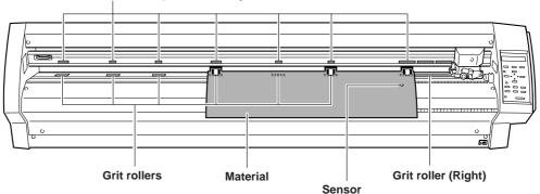
Load the material so that it lies over the sensor on the platen.
