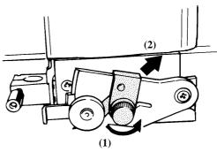
\* If the blade remains in the carriage, use tweezers to remove it.
