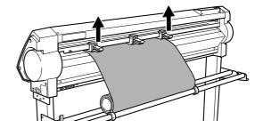
Position the stoppers so that they lightly touch the edges of the roll and secure in place by tightening the screws so that the roll material does not move from side to side during material feed.
