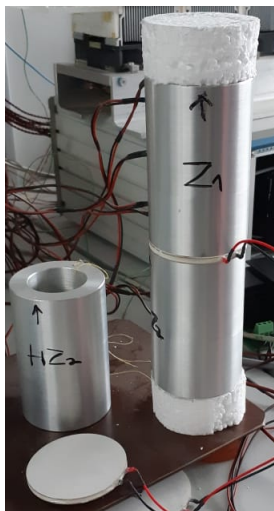
Fig. 8 Experimental setup: a thin Peltier element b/w two aluminum cylinders. The cylinders are thermally insulated at the ends, the temperature is measured at several points on cylinders' sides.
