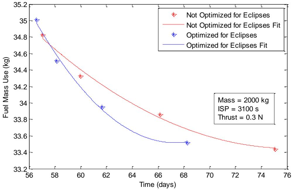
**Figure 9. Maneuver Time vs. Propellant Mass Consumption Optimized and Not Optimized for Eclipse Periods**
