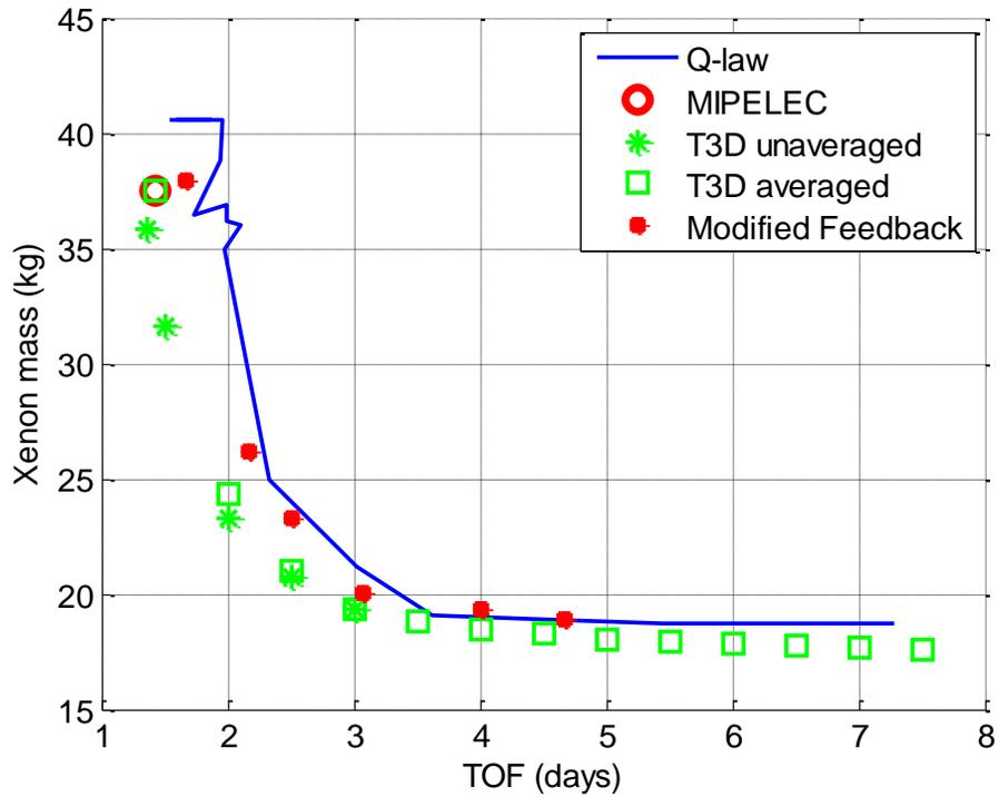
Figure 6. Fuel mass consumption vs. time-of-flight for Case C
