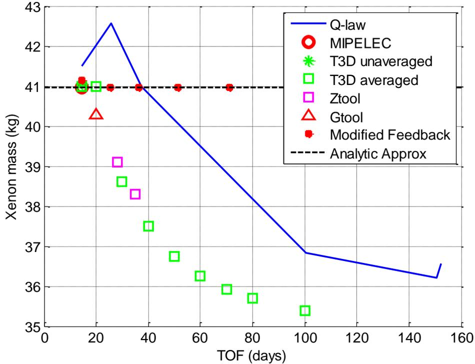
**Figure 4. Fuel mass consumption vs. time-of-flight for Case A, comparing existing tools (compared in reference 1) to the modified feedback control and analytical approximation**
