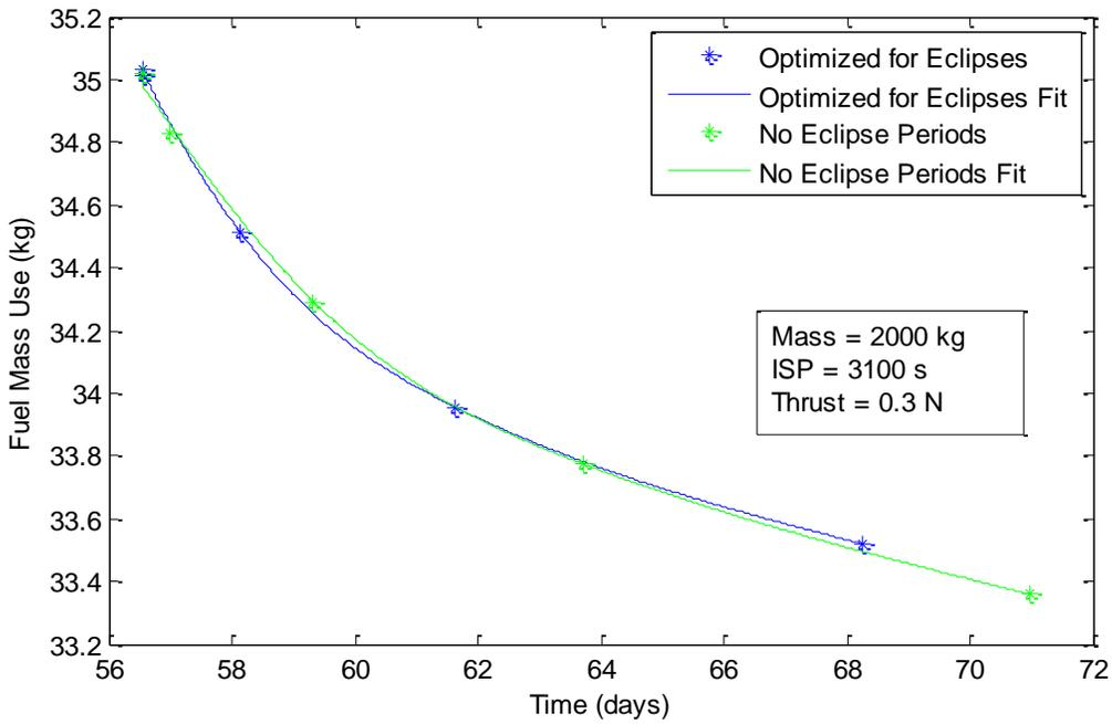
**Figure 10. Maneuver Time vs. Propellant Mass Consumption Optimized for Eclipse Periods and Without Eclipse Periods**
