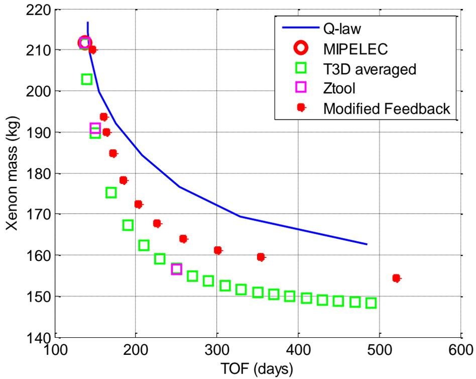
Figure 5. Fuel mass consumption vs. time-of-flight for Case B
