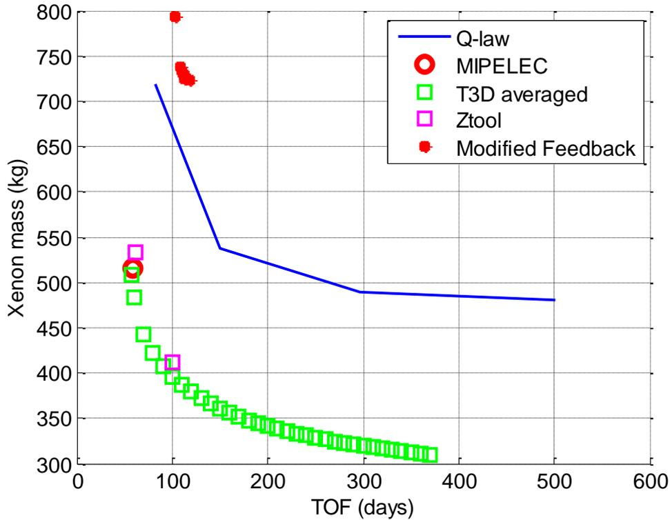
Figure 7. Fuel mass consumption vs. time-of-flight for Case E
