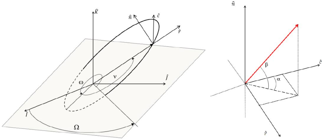
**Figure 1. Left: RCN reference frame with respect to the Central-Body-Centered inertial reference frame (IJK). Right:  $\alpha$  and  $\beta$  thrust angles with respect to the RCN reference frame.<sup>3</sup>**
