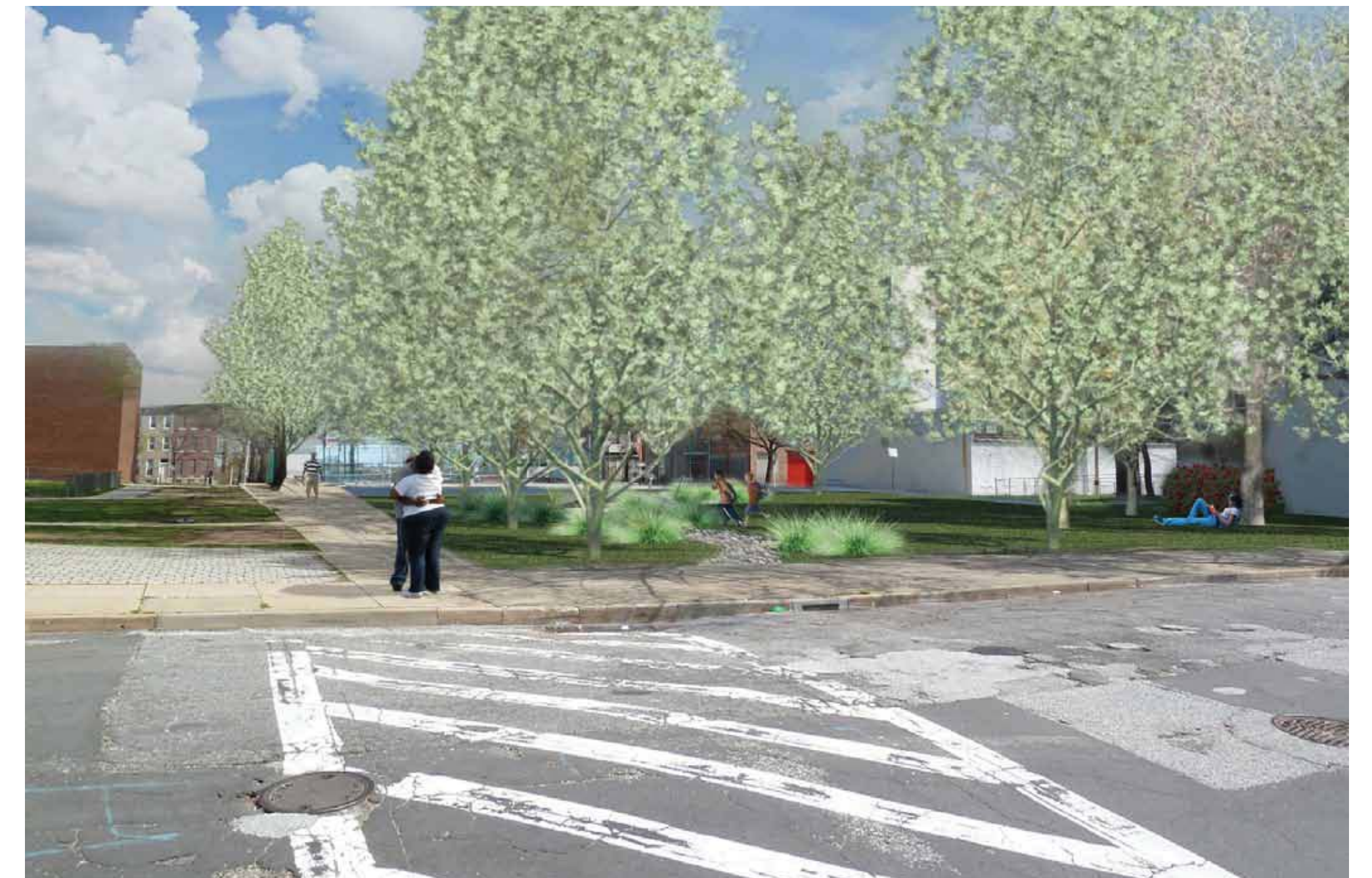
The dry stream bed will be incorporated into Oliver's Neighborhood park to continue the visible stormwater trail, act as an educational tool for schools adjacent to the site, and cleanse stormwater running into the park from East Hoffman Street.
