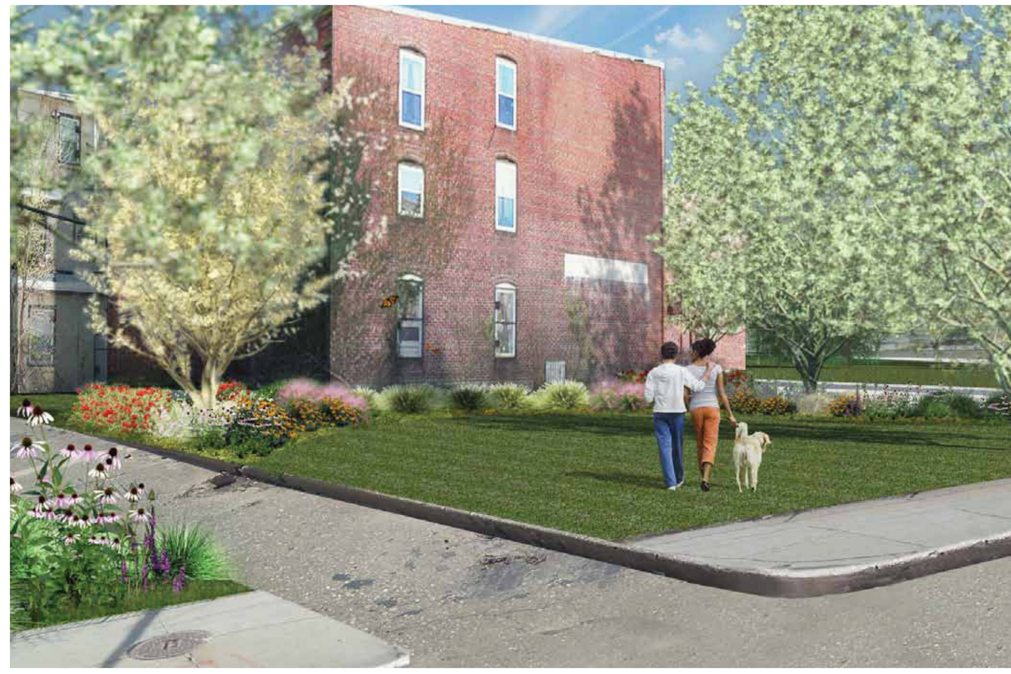
RAIN GARDEN NEAR HOUSE OF GOD IN CHRIST FOR ALL Water flowing from the roof of the church, as well as stormwater running onto the site, flows into the rain garden located on this particular vacant lot. Since the soils within the Oliver Neighborhood have a low-infiltration rate, a layer of gravel and a perforated pipe are included to convey excess water off of the site. Excess water may also follow the visible trail by flowing across Hubbard Alley underneath a metal grate and into another rain garden located on the adjacent lot.
