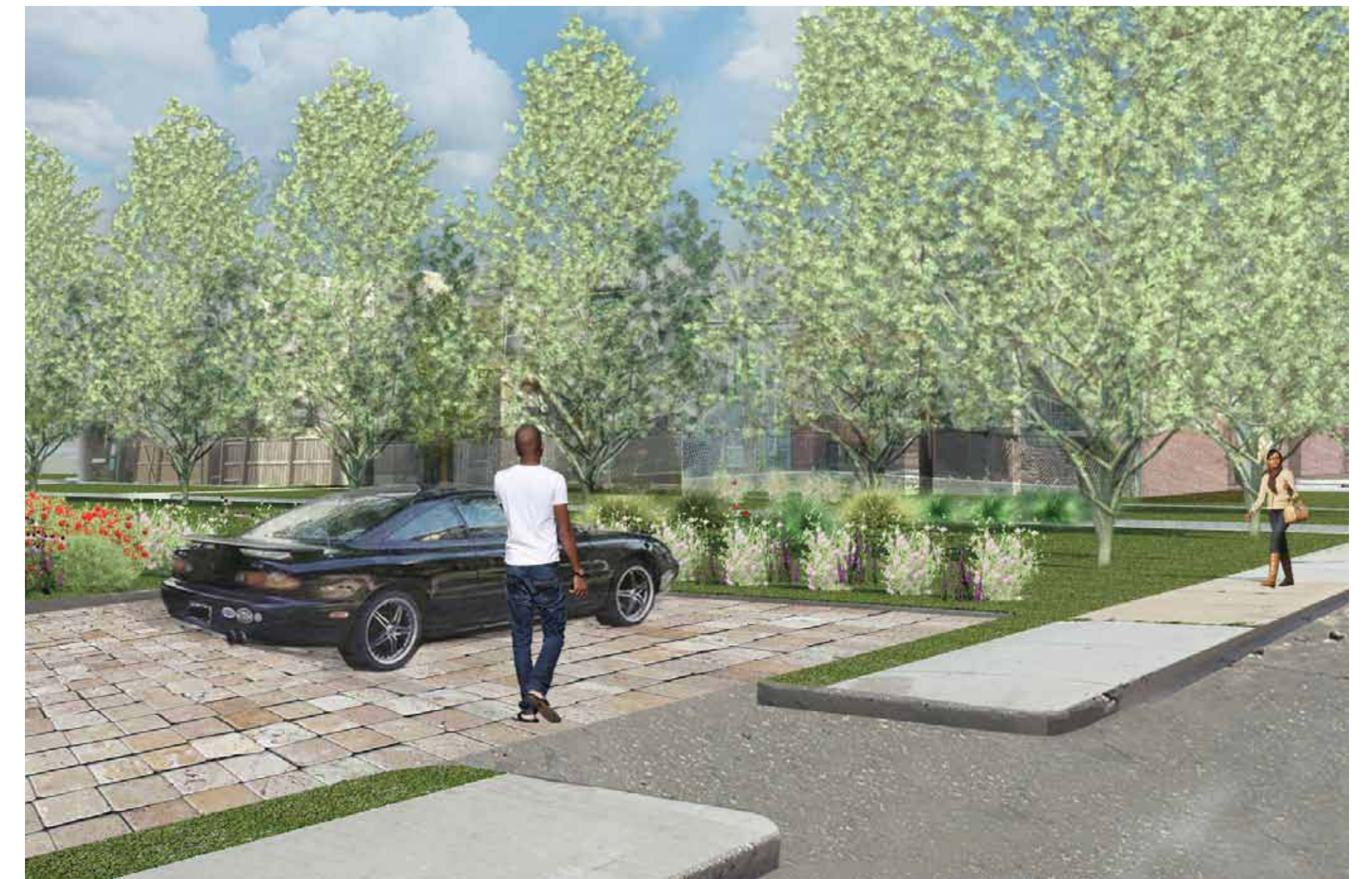
A stainless steel linear runnel allows water to flow across one vacant lot, underneath a drainage trench, and into a bioswale near the existing parking lot located on site. Permeable pavement will replace the existing pavement to help infiltrate stormwater runoff that runs along east hoffman avenue before entering the bioswale.
