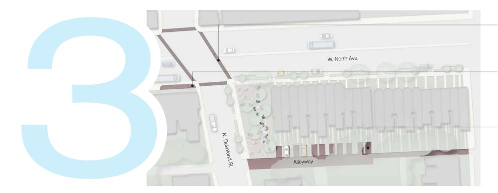
The final phase in this "check" point design project will be to repave the existing bus stop at the corner of W. North Ave., pedestrian crosswalks that stretch across W. North Ave. and N. Dukeland St., and the alleyway connecting N. Dukeland St. and Ashburton St. These additions will help will stormwater runoff collection, pedestrian safety, and visual connections to the repurposed vacant lot.
