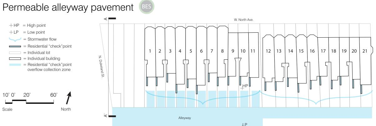
*The permeable pavement* added to the alleyway connecting N. Dukeland St. and Ashburton St. will allow the overflow roofwater running from the adjacent row homes to collect and infiltrate into the ground. There it will be cleansed and introduced into the existing stormwater system
