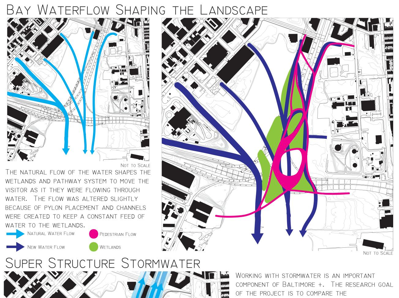
IS POURED INTO THE BAY VERSUS TREATING IT IN BRIDGE WATERFLOW HAD TO BE UNDERSTOOD. THE WATER FLOWS NOT ONLY WITH THE SLOPE OF THE CONCENTRATION IN THE CURVES OF THE ROADS. THIS REVEALED IMPORTANT POINTS OF INTEREST TO CONSIDER TESTING PRE-TREATMENT.
