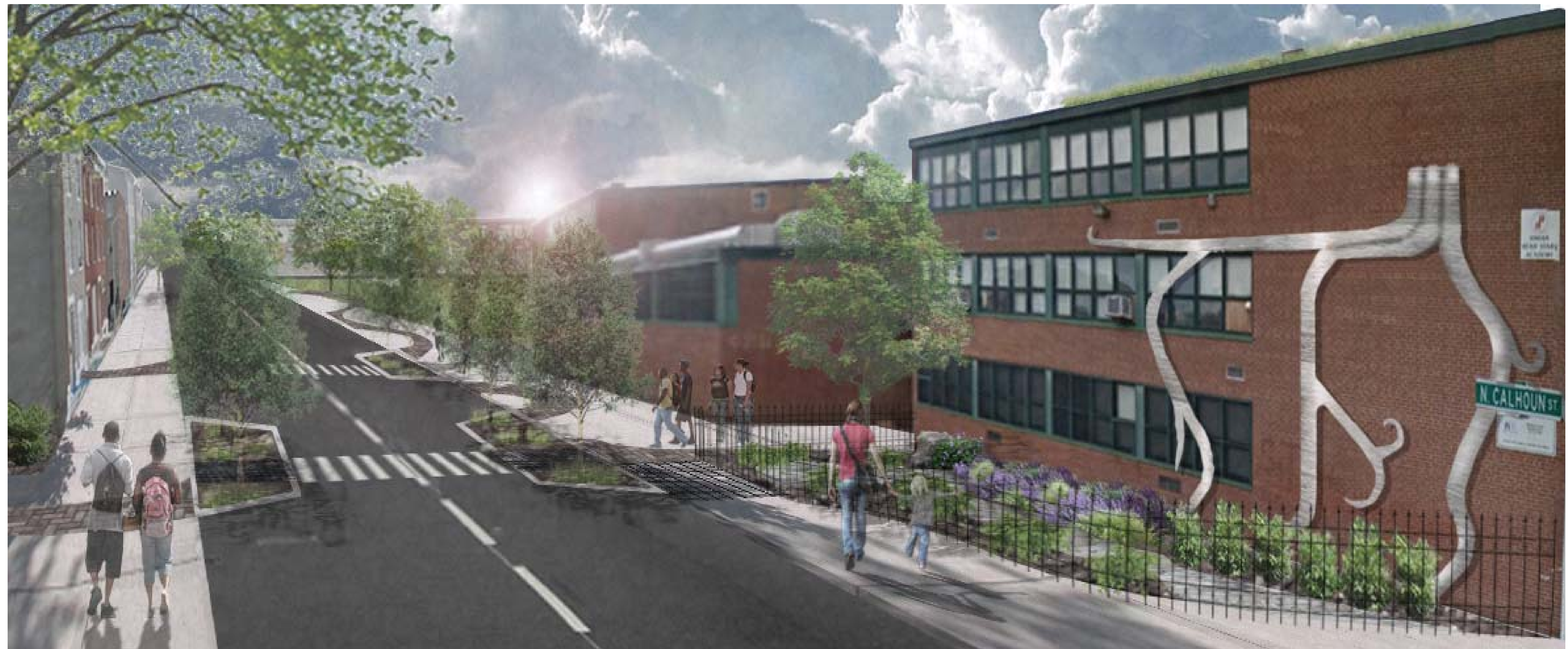
This rendering shows Phase II in its completion: the artful stormwater garden that gathers runoff from the roof through artful piping, multiple curb expansion stormwater gardens that capture runoff from North Calhoun St., and artful permeable pavement. Maintenance of the artful stormwater garden can be accomplished by school staff and if willing the students, too. The maintenance of the curb extension stormwater gardens will be the city's responsibility.
