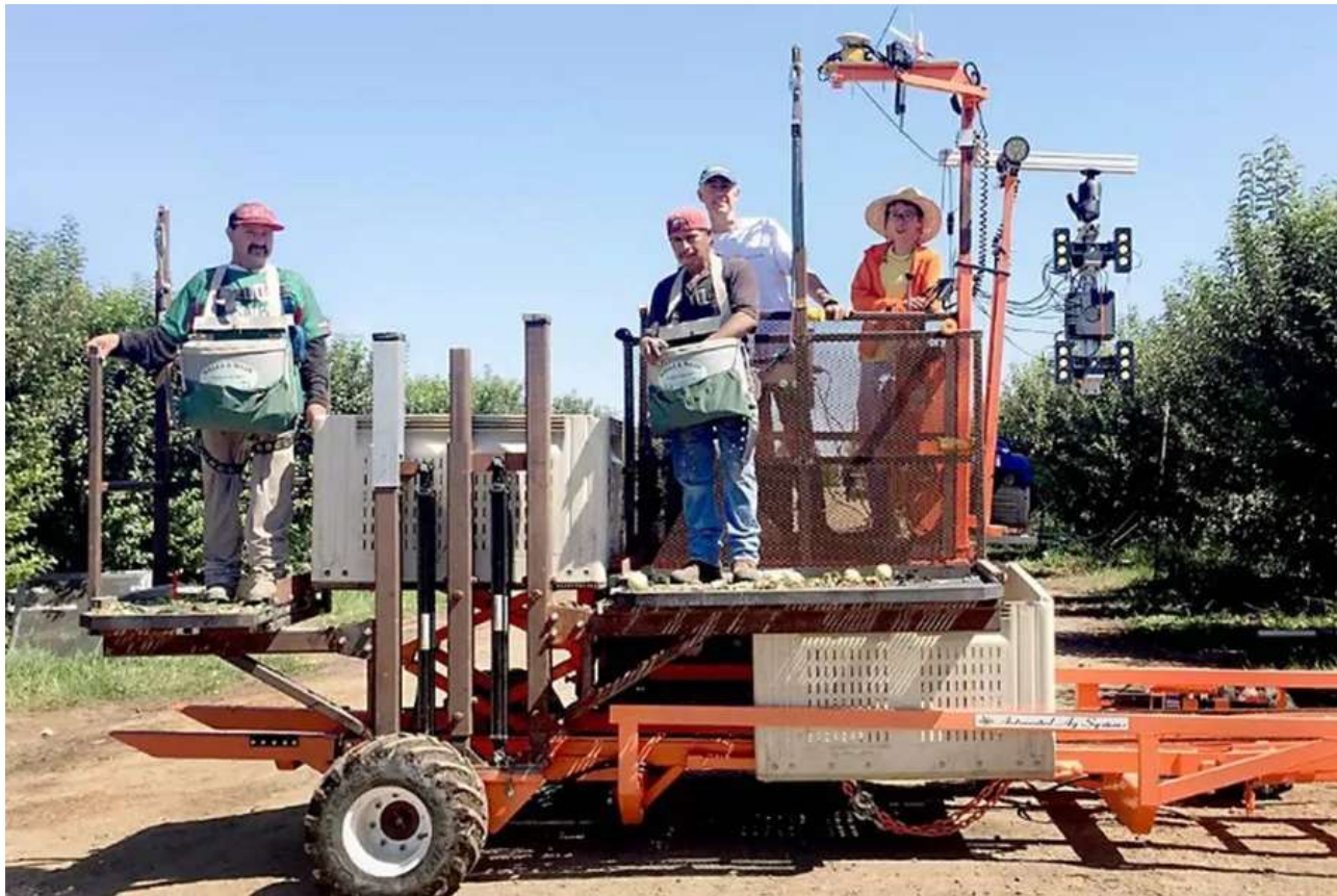
Figure 2. Apple harvest-assist platform based on fruit distribution by a machine vision system (University of California, Davis).
