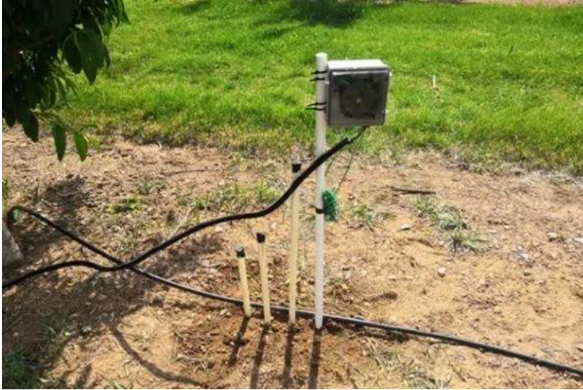
Figure 1. A soil moisture sensor-based irrigation system in a peach orchard. Image: Long He, Penn State
