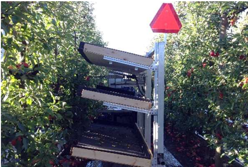
A multi-tier shake-and-catch harvesting platform (WSU design by Dr. He and team).
