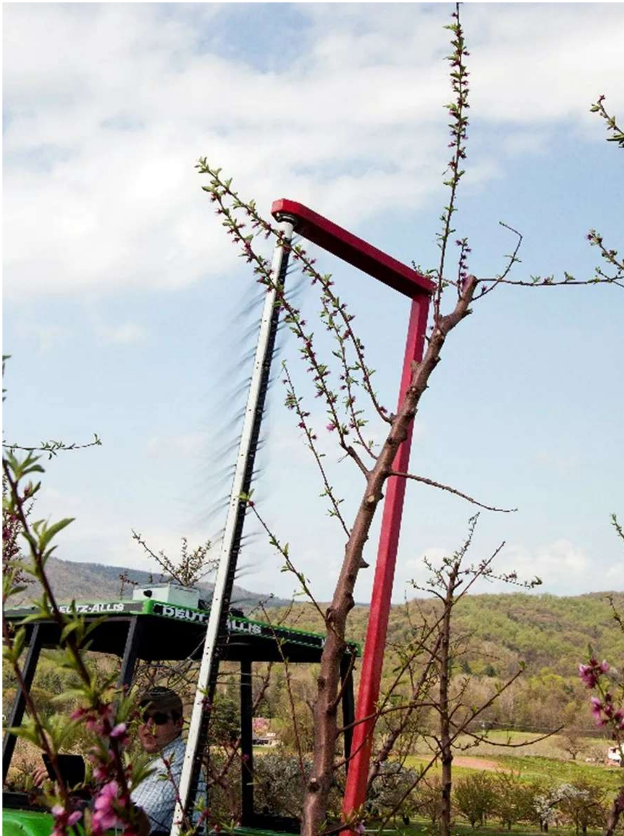
Mechanical peach blossom thinner commercialized as a result of multi-state research led by Penn State. Photo: Loy Elliott
