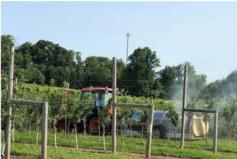
Figure 1. An air blast sprayer in operation at the Fruit Research and Extension Center (FREC) orchards in Biglerville, PA. Photo: Long He, Penn State
