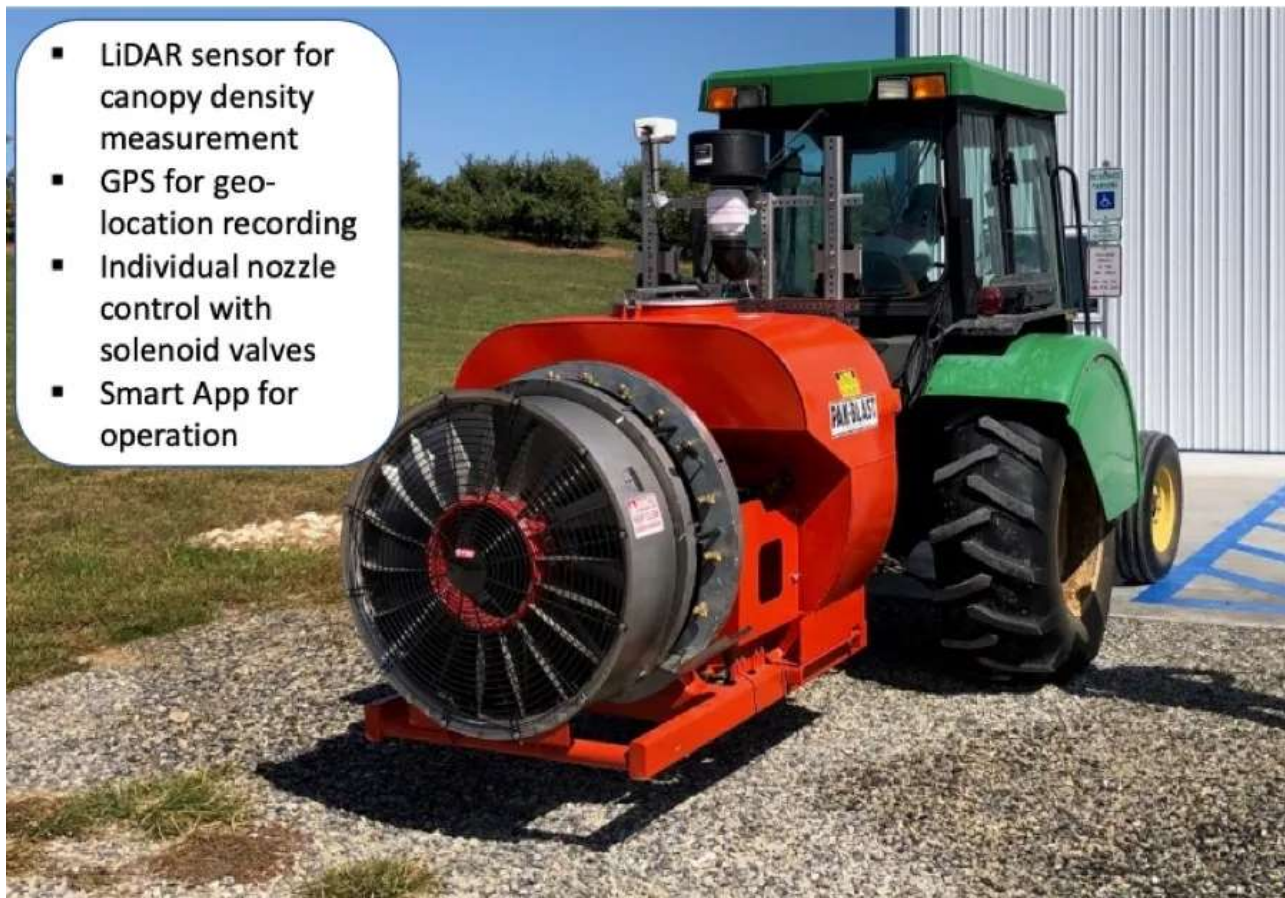
Figure 3. A LiDAR-guided precision sprayer attached to a tractor. Image: Long He, Penn State
