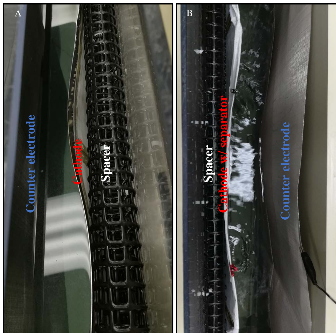
Figure S1. Photos of the plastic spacers in the large chamber (A) in the absence and (B) in the presence of a separator.
