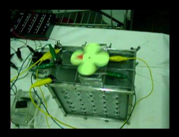
MFC webcam (live video of an MFC running a fan) www.engr.psu.edu/mfccam
