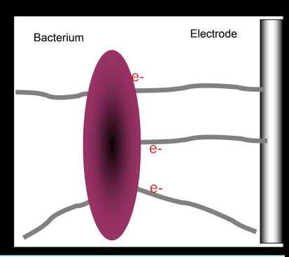
Bacteria that can transfer electrons directly to the electrode:
