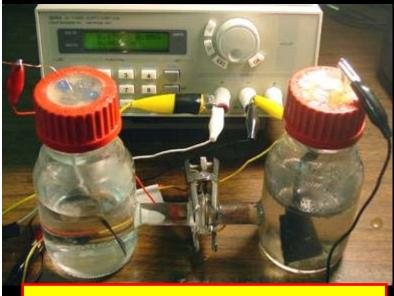
BEAMR voltage much less than that needed for water electrolysis (1.8 V)
