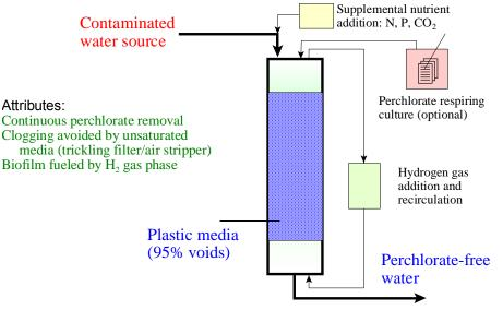
Hydrogen-oxidizing, autotrophic, perchlorate reduction is possible
