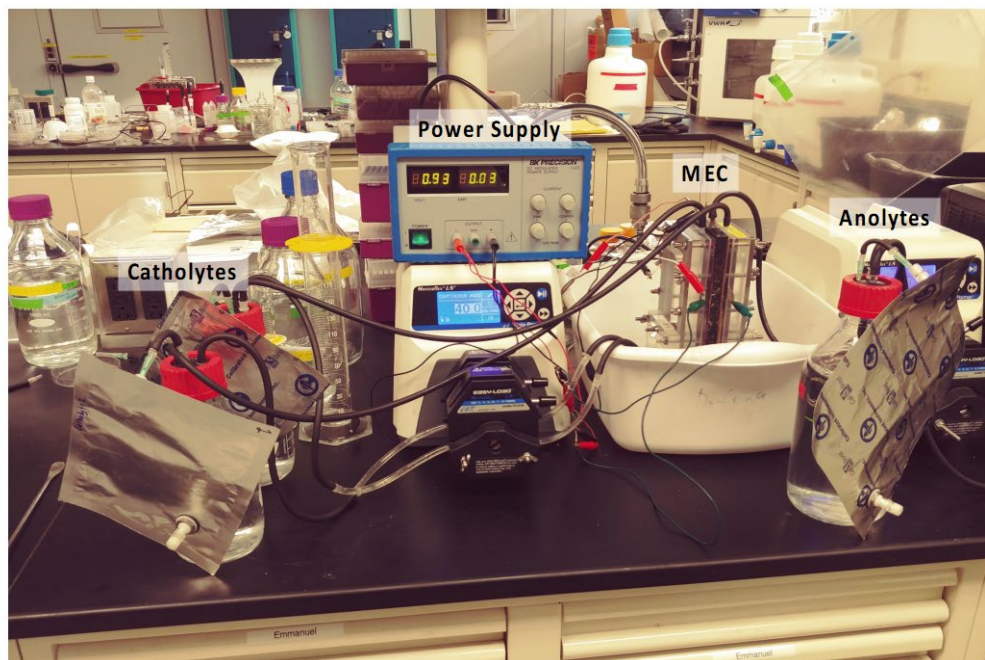
Fig. 2. The setup for operation of the single 5.5 cm diameter graphite brush anode MEC.
