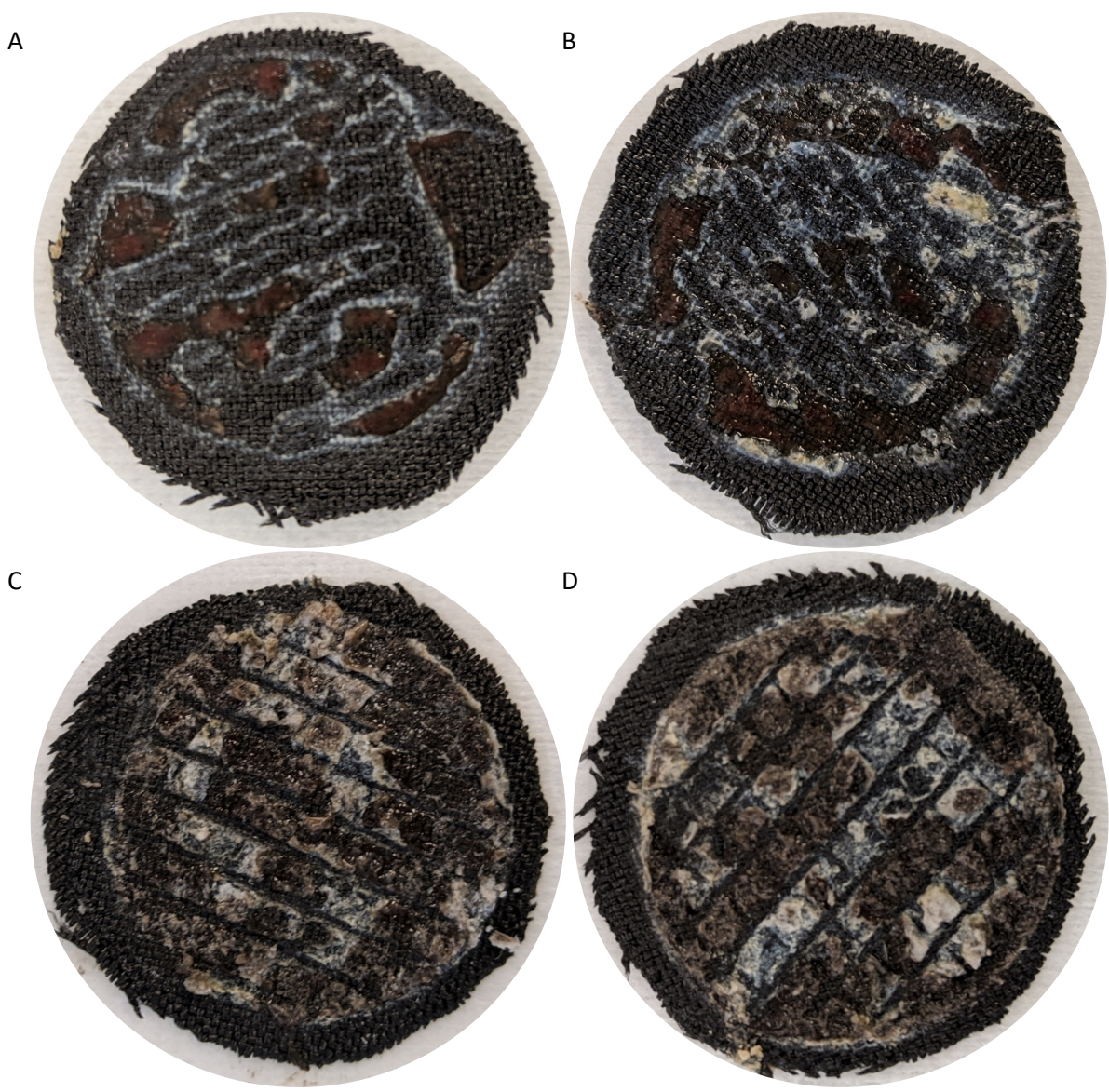
Figure S11: Photos of the (A, B) cathode side and (C, D) plastic spacer side of the carbon cloth anodes from duplicate reactors after 35 days of operation.
