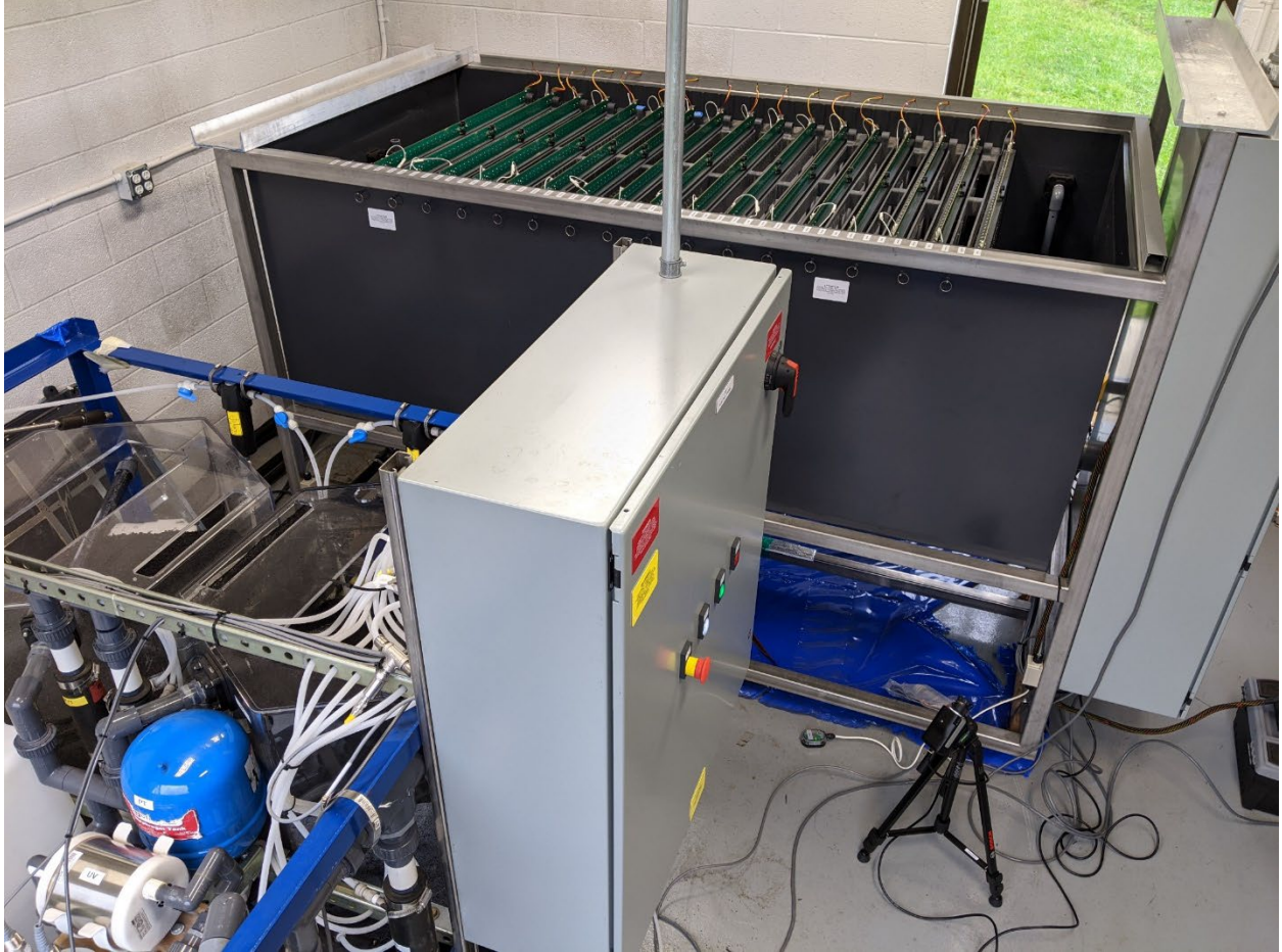
Figure S7. Photo of the combined MFC/BF skid. The wastewater was flowing by gravity from the MFC to the BF.
