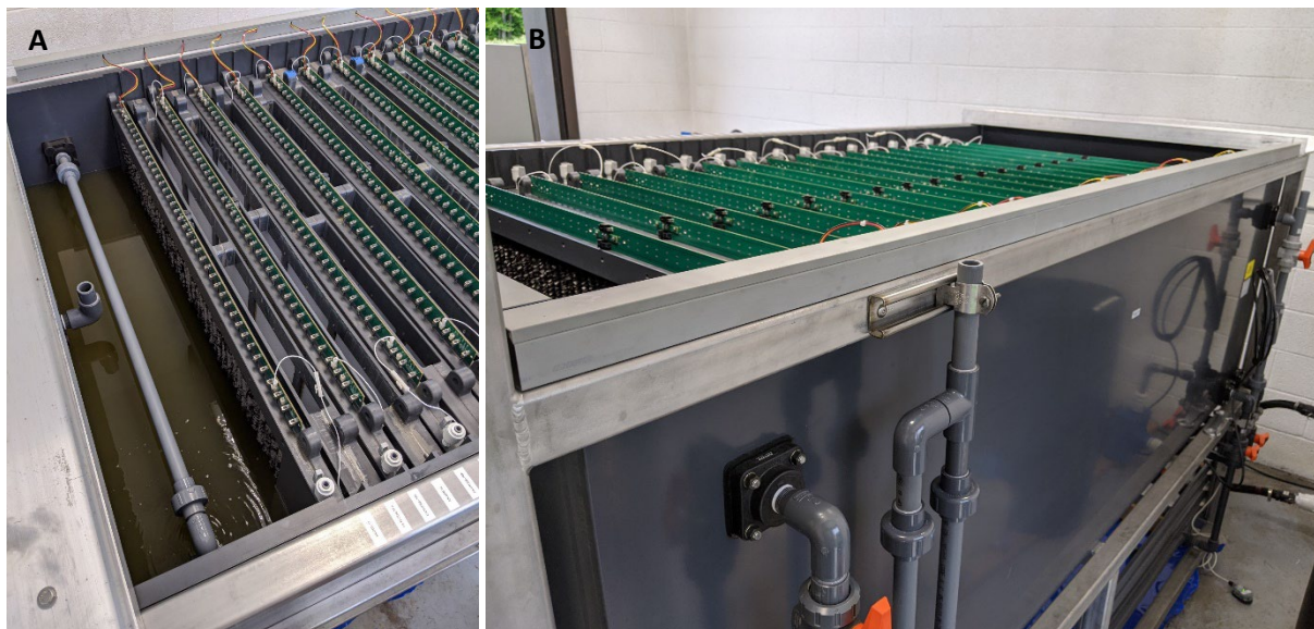
Figure S5. Photos of the MFC during operation. (A) Photo of the influent section and (B) of the side of the tank.
