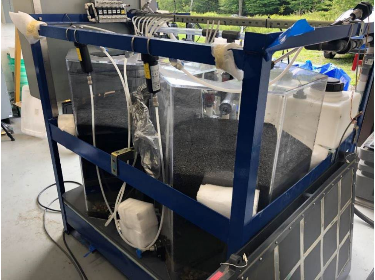
Figure S3. Close-up photo of the two GAC tanks of the BF unit.
