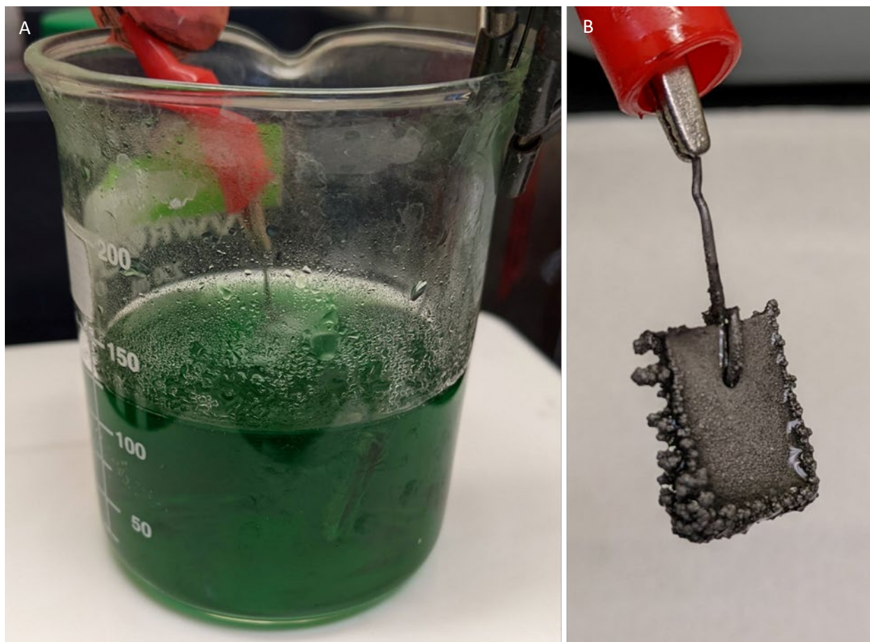
Figure S1. NiMo Elec synthesis. (A) Photo of the cell configuration for the NiMo Elec preparation and (B) photo of the deposited NiMo on the graphite block. The NiMo Elec was collected from the bottom of the beaker and gently scraped from the graphite block before being washed, dried, and analyzed with XPS.
