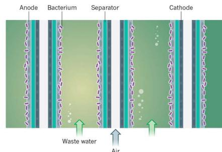
Figure 3 | An MFC stack. MFCs are arranged close together to reduce internal resistance and form compact reactors. Within the stack the electrodes consist of repeating units of an anode coated in a mat of bacteria, or biofilm, an insulating separator and a cathode. Waste water flows over the anodes and air over the cathodes. The individual anode and cathode are connected by a wire (not shown).
