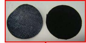
Activated carbon cathode works almost as well as Pt catalyst
