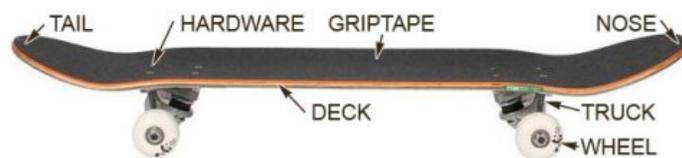
**Figure 1 Photo of a Skateboard:** Basic parts of a skateboard
