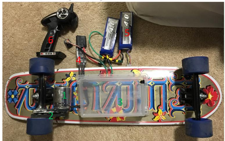
**Figure 2 Photo of an Electric Skateboard:** Additional components used to create an electric skateboard. Numbers used in image correspond to component list to the left of the image. Mechanical parts are labeled in green, while electrical parts are labeled in red.
