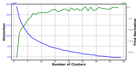
Fig. 19: The result of elbow method on the dataset. We could spot the elbow around 13-17 clusters. We are also showing the first derivative of the distortion, to show where it is going to flatten out.
