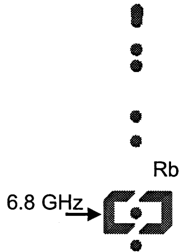
Figure 11. Juggling pattern of alternate launch delays of 22 and 55 ms to cancel the s-wave juggling frequency shift.
