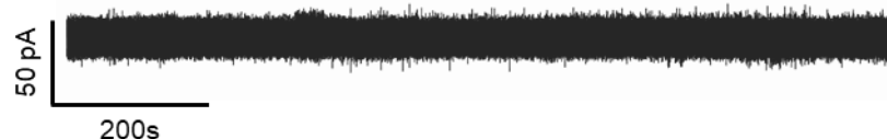
Figure 4-3. Nanopore experiment for a pure RNP and HIV targets sample (30 nM) without any ssDNA reporter. We did not observe a single event for a measurement duration time of 1000 s, which confirms that the translocation rate of the background activated RNPs is less than 0.001 \text{ s}^{-1} .
