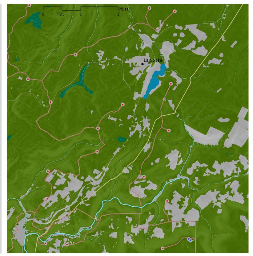
Although the majority of focus on Marcellus impacts revolves around the well itself and the well pads they operate on, the access roads and gathering pipelines play a significant part in land planning and design issues. The corridors cut through the landscape causing visual and physical changes to the landscape.
