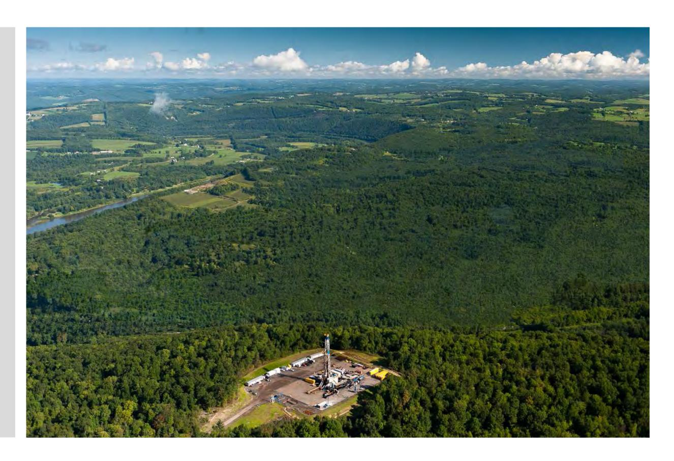
Although the equipment has been cleared off of the lower well pad, it is still in production. The drill rigs are only in operation at the start of the well's life in order to drill, frack, and start the extraction process. Well pads will look like this throughout their operational lifespan.
