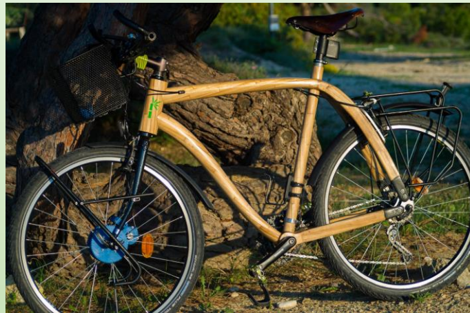
Figure 1. Bicycle model with a frame made of bamboo composite (Soben Advanced Bamboo Composites, 2019)
