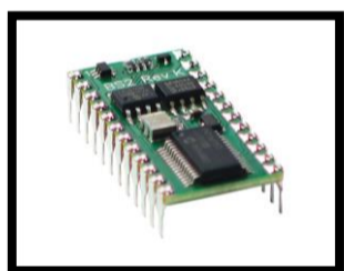
Figure 1. BASIC Stamp 2 is a programmable microcontroller. It can control and monitor timers, keypads, motors, sensors, switches, relays, lights, and more [1].
