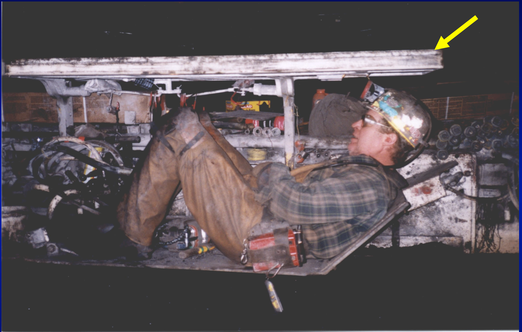
TRAM STATION CANOPY ON LOW-COAL ROOF BOLTING MACHINE
