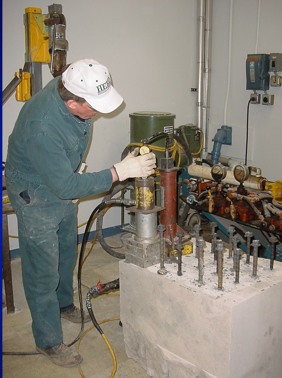
Resin Anchorage Test
