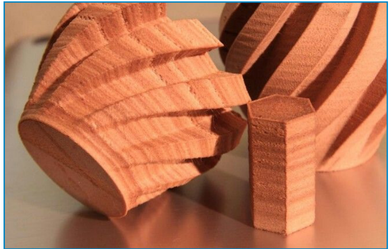
Wood Polymer Filament: A PLA filament infused with wood particles. Used to create decorative objects where the appearance and feel of wood has sensory importance.
