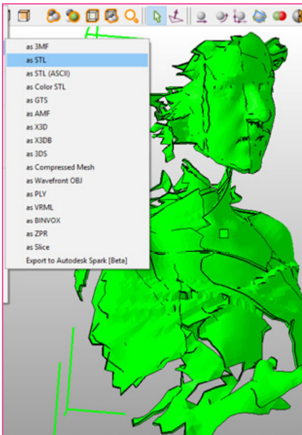
Figure 1. Repaired glitchy 3-D digital model being exported into a STL file for printing.
