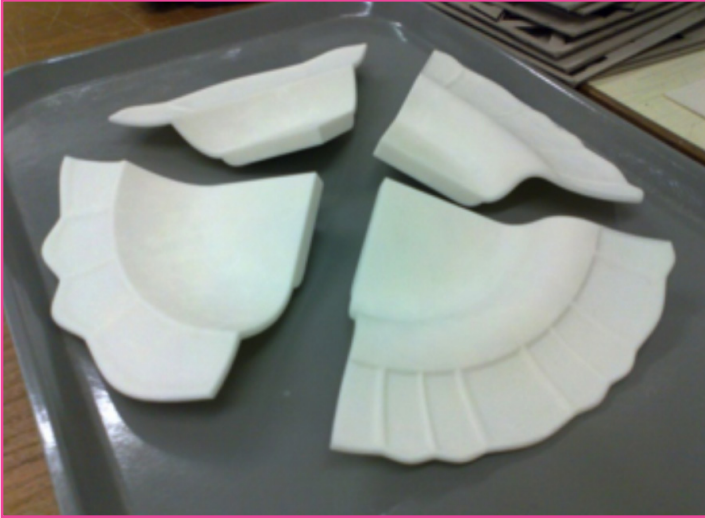
Figure 2 - 3-D printed prototypes of designs generated by the Grasshopper design system.
