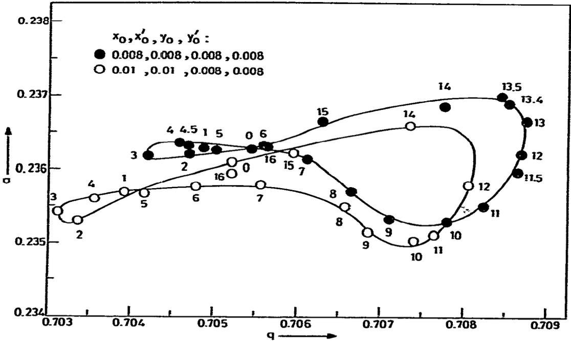
Fig. 2. Practical stability diagram apex point loci due to initial phase  $\xi_0$  variation. The circles represent apex points from actual computation for specific initial phases; the  $\xi_0$  values are shown next to the circles in units of  $\pi/16$ . The locus between the open circles for  $\xi_0 = 12(\pi/16)$  and  $\xi_0 = 14(\pi/16)$ , in the absence of information on  $13(\pi/16)$ , is somewhat uncertain.
