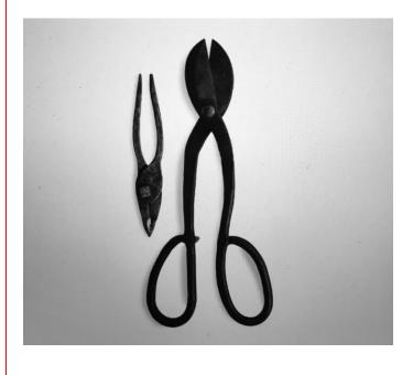
**Figure 34:** *"Tin Snips and Pliers"* – A plier (left) and tin snip (right) made from molten scrap metal by Akira Oye, a Japanese American interned at a camp in Rohwer, Arkansas. Tools such as these were often made melting down scrap metal in a boiler furnace and then hammering it out into a desired shape.
