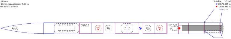
Apogee: 5298 ft 682 ft/s (Mach 0.61) Max. velocity: Max. acceleration: 302 ft/s<sup>2</sup>
