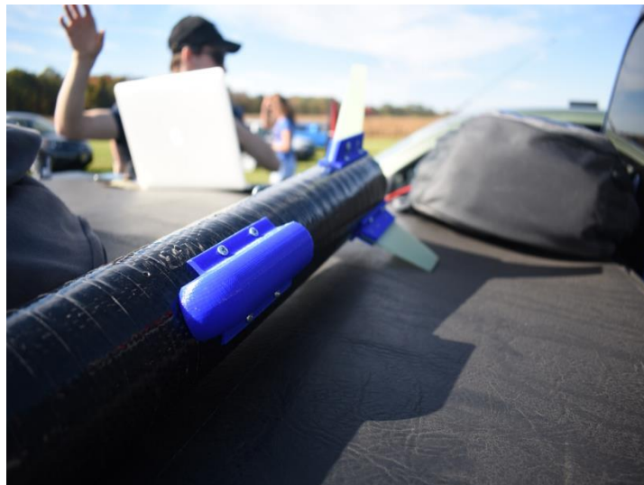
Figure 2. Refined camera cover design on subscale rocket (3" body tube)
