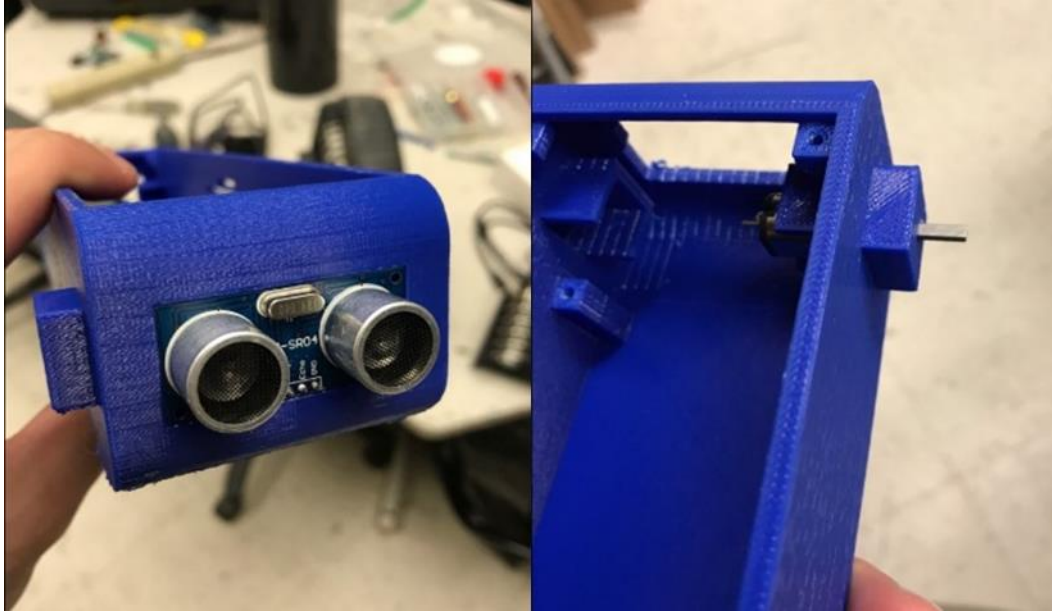
Figure 29. Ultrasonic sensor (Left), Installed motor (Right)
