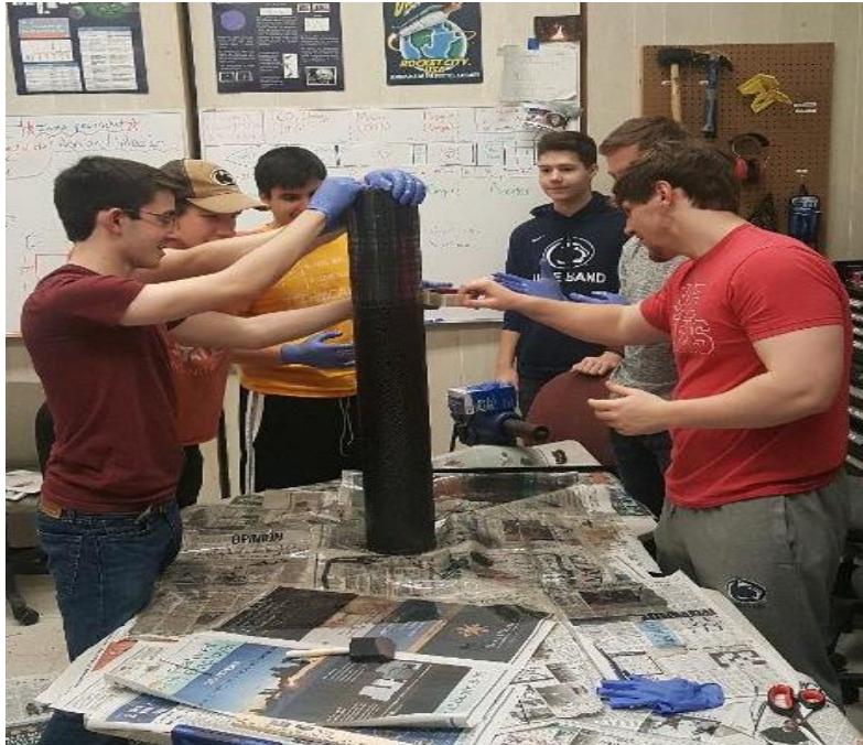
Figure 2. Wrapping the carbon fiber blue tube in heat shrink tape
