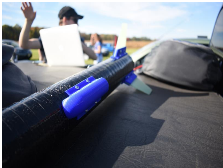
Figure 3. Refined camera cover design on subscale rocket (3" body tube)
