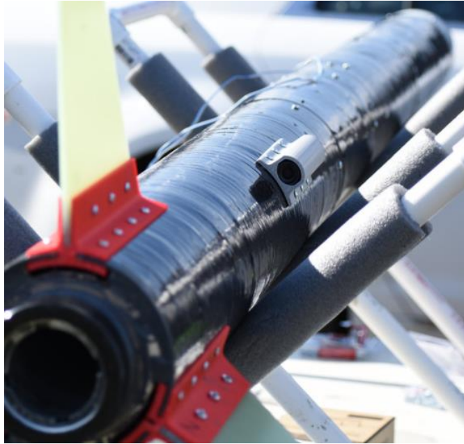
Figure 4. Camera cover design on fullscale rocket (5.61” outer diameter body tube)
