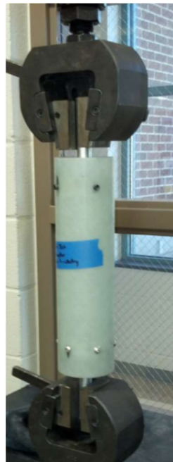
Figure 5: Tensile Testing Setup for G12 Fiberglass Specimen
