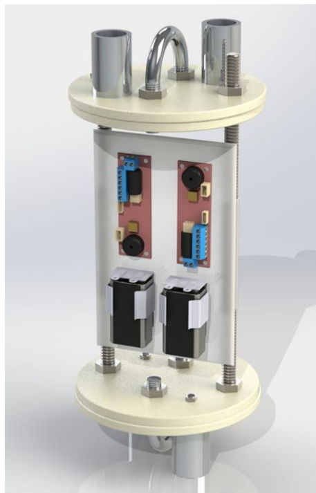
Figure 5: Avionics bay preliminary layout with fiberglass board
