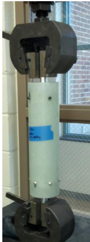
Figure 35: Tensile Test Setup for G12 Fiberglass Specimen
