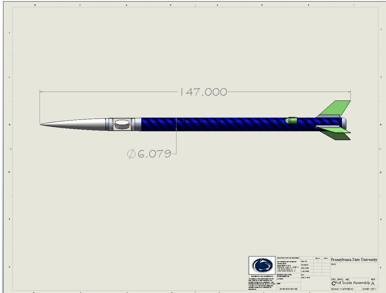
Figure 5: Dimensioned Drawing of the full-scale Vehicle Assembly
