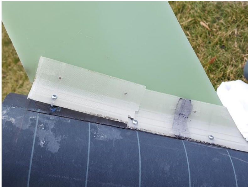
Figure 29: Damaged fin bracket
