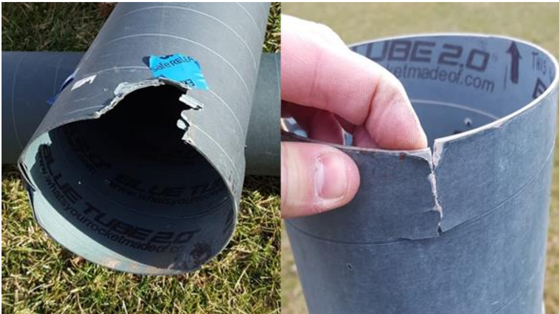
Figure 28: Zippering of main body tube (LEFT) and booster coupler (RIGHT)
