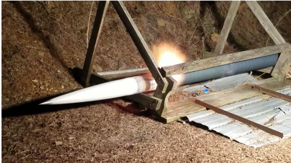
Figure 42: The moment of detonation during a main parachute deployment test
