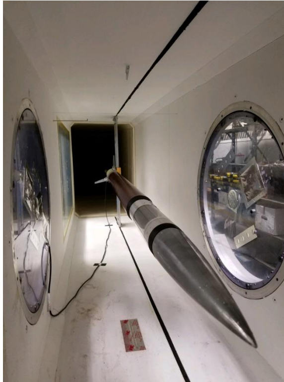
Figure 39: Sub-scale rocket mounted in Laminar Flow wind tunnel
