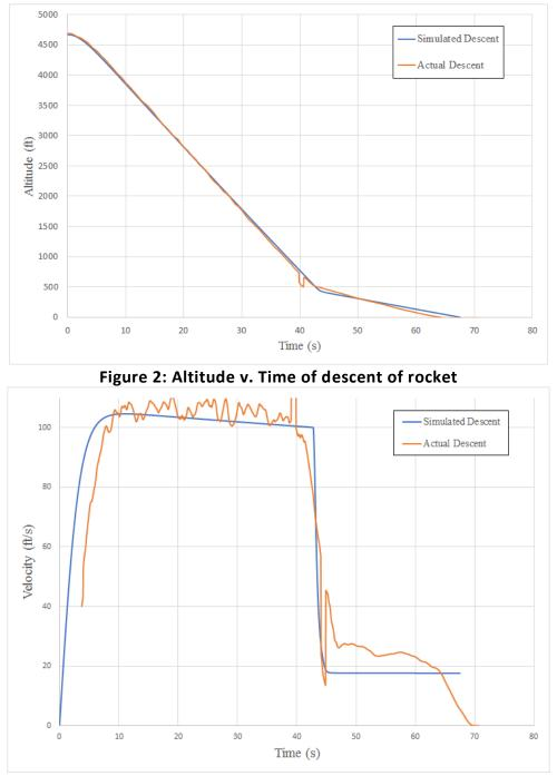
Figure 3: Velocity v. Time of Rocket During Descent
