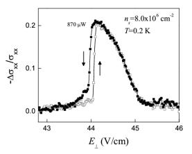
many-electron optical bistability – observed in the 2D world only for e-on-He, Konstantinov et al.
