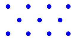
Bragg-Cherenkov many-electron friction: where the ripplon frequency  $\omega(G) = \mathbf{v} \cdot \mathbf{G}$ , all ripplons are emitted in phase The force on the Wigner crystal  $\propto N^2 \implies$  "many-electron sound barrier"
