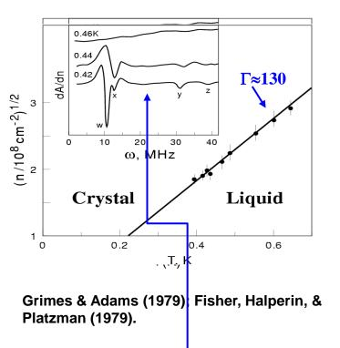
Resonances at the frequencies of capillary waves with **q=G**, reciprocal lattice vectors
