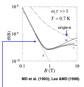
Short-wavelength scattering by capillary waves with the momentum transferred to the electron liquid. **Instead of quantum Hall!**
