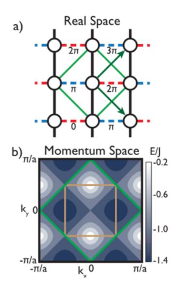
Super-strong magnetic field One half flux quantum per unit cell
