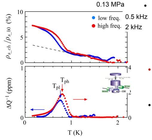
The rapid growth and the dissipation peak shift to low temperature by ~40 mK.
