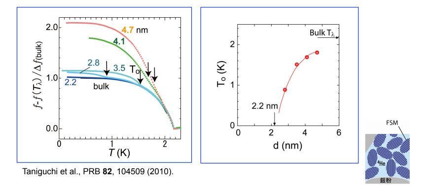
A clear rise due to the superfluid response in the channel is observed above 2.8 nm in addition to the bulk one.
