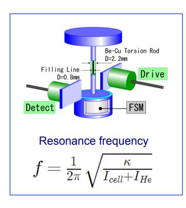
Superfluidity of <sup>4</sup>He in 1D channel was measured by means of a torsional oscillator.
