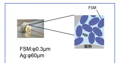
Pellets were prepared by sintering FSM16 and silver powder.
