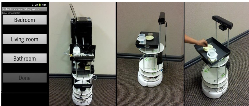
Fig. 1 A water and medication delivery robot. Users requested service from the robot by pressing a button on their smart phone indicating their location. The robot then traveled to a medication and water station for pickup of the items to be delivered, traveled to the stated location, and stopped within an arm length of the person.
