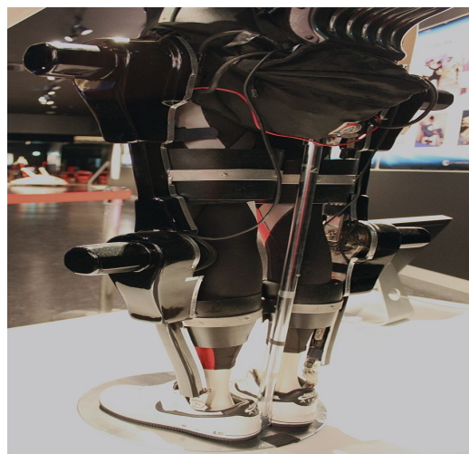
Figure 1 An exoskeleton platform for human mobility enhancement. Exoskeletons enhance the patient's mobility by providing additional battery powered strength to one's joints and by enhancing one's balance. The exoskeleton photograph is by Yuichiro C. Katsumoto from Shonan, Japan-Cyberdyne Studio. Uploaded by Chime, CC BY 2.0, commons.wikimedia.org/w/index.php?curid=9963050.
